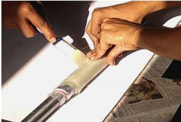
Fig.1: Fabrication of FML cylindrical structure using pultrusion technique
