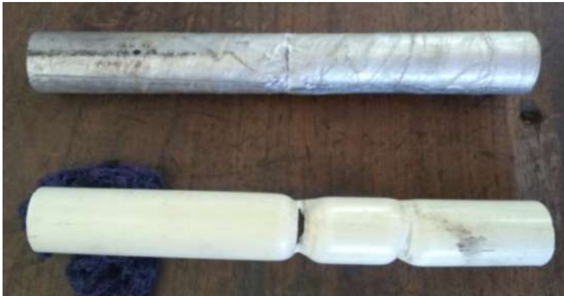
Fig. 3: FML (top) & PVC (bottom) pipes after buckling failure
