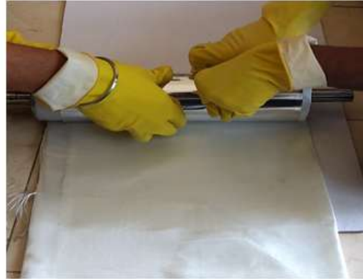
Fig. 2: Rolling up of sandwich FML composite on the cylindrical mould
